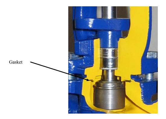
Everytime when valve bonnet was disassembled sealing surface should be cleaned. During assembly it should be applied new gasket of the same type as previously used. Body-bonnet bolt connections should be tighten when the valve is at open position. The bolts should be tighten evenly and crosswise by torque wrench.
