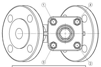
Tighten sequence of body – cover bolt nuts
