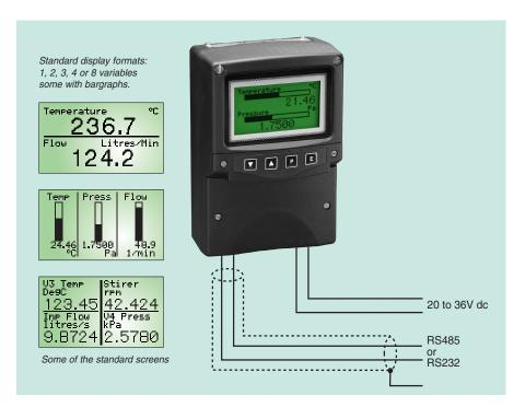
The BA684D is a dc powered instrument that can display text and simple graphics in a process area. Incorporating four pushbuttons and two single pole outputs, the BA684D is a low cost robust operator interface ideal for simple machine and process control applications.
