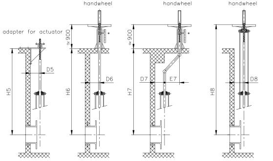
5) Rising stem with wall support and adapter for actuator
