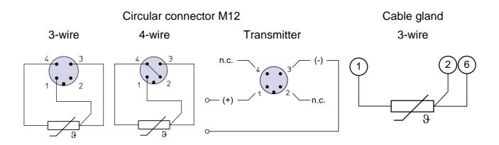
Figure 1: Variants of electrical connection
