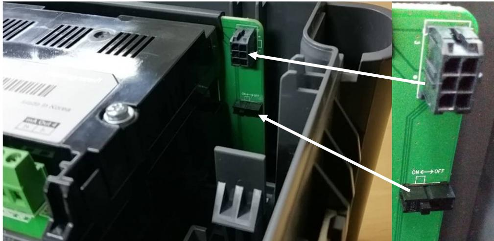
Figure 37. Battery On/Off Switch and Battery Connector
