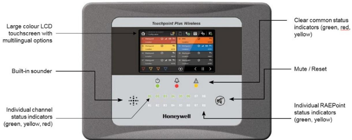
Figure 35. Touchpoint Plus Wireless Controller User Interface
