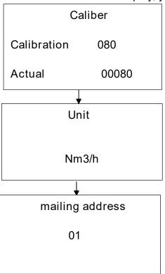
Under the language menu, press to save and enter the caliber menu. Press to save and go to the next menu, press to move the cursor position, and to modify the parameters.
