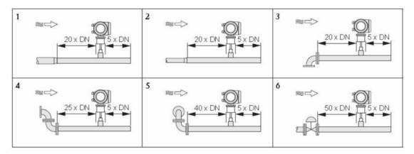
1 = Reduction, 2 = Expansion, 3 =  $90^{\circ}$  elbow or T-piece, 4 =  $2 \times 90^{\circ}$  elbow, 5 =  $2 \times 90^{\circ}$  elbow (3-dimensional), 6 = Control valve or pressure regulator.
