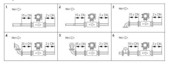
1 = Reduction, 2 = Expansion, 3 =  $90^{\circ}$  elbow or T-piece, 4 =  $2 \times 90^{\circ}$  elbow, 5 =  $2 \times 90^{\circ}$  elbow (3-dimensional), 6 = Control valve.
