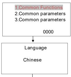
In the main interface, press to enter the main menu interface. You can use the shift keys to select the corresponding menu item and press set to enter.
