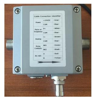
Fig. 5.1 Cable Connection Identifier
