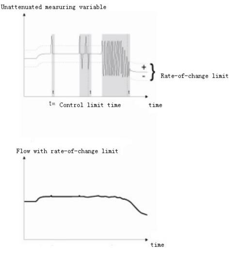
Fig.6.2 Example for the effect of rate-of-change limit
