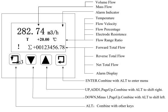
Fig. 6.1 Keypad and LCD for Display version
